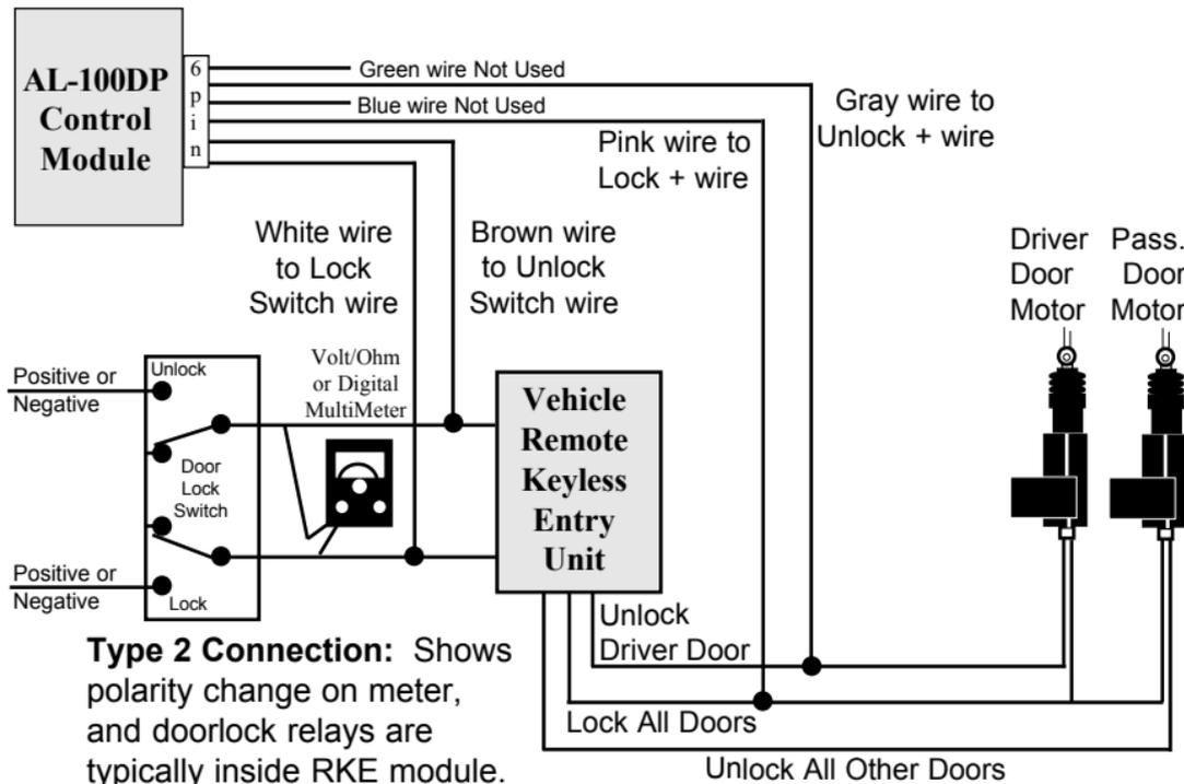
**Type 2 Connection:** Shows polarity change on meter, and doorlock relays are typically inside RKE module.
