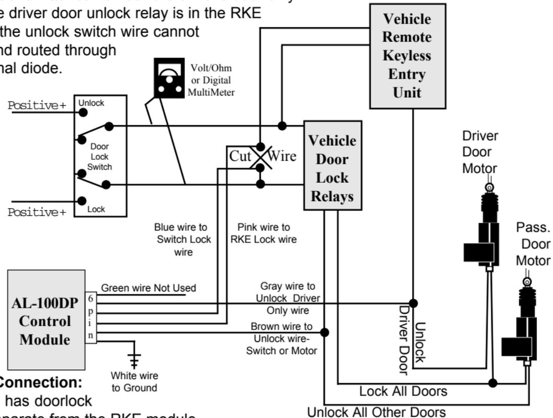
**Type 3 Connection:** Typically has doorlock relays separate from the RKE module.
