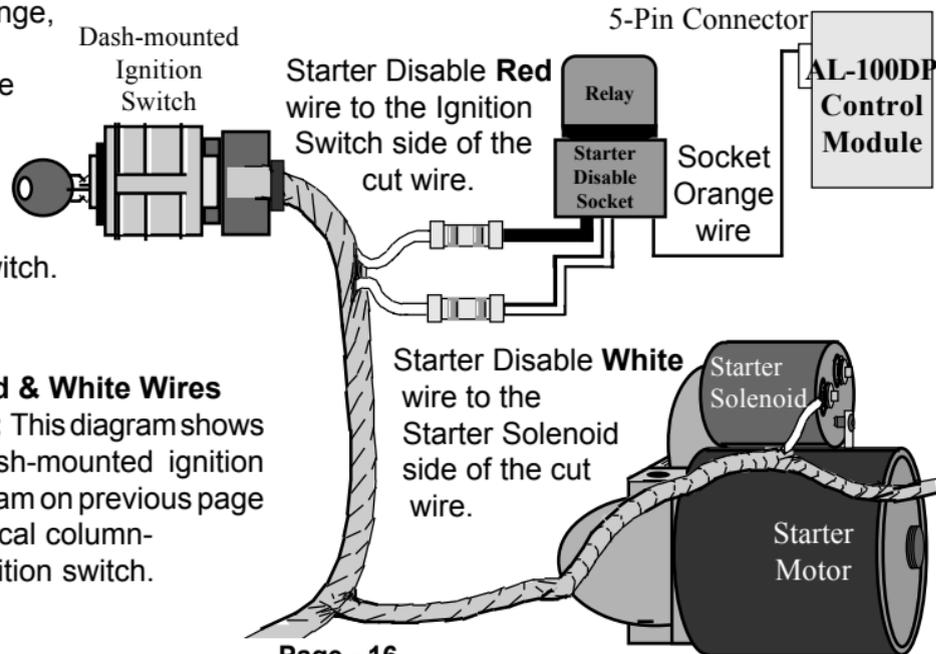
**Orange, Red & White Wires Connection:** This diagram shows a typical dash-mounted ignition switch; diagram on previous page shows a typical column-mounted ignition switch.
