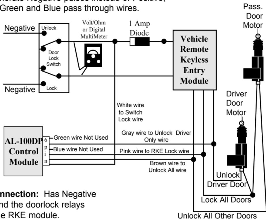
**Type 4 Connection:** Has Negative switches and the doorlock relays built into the RKE module.
