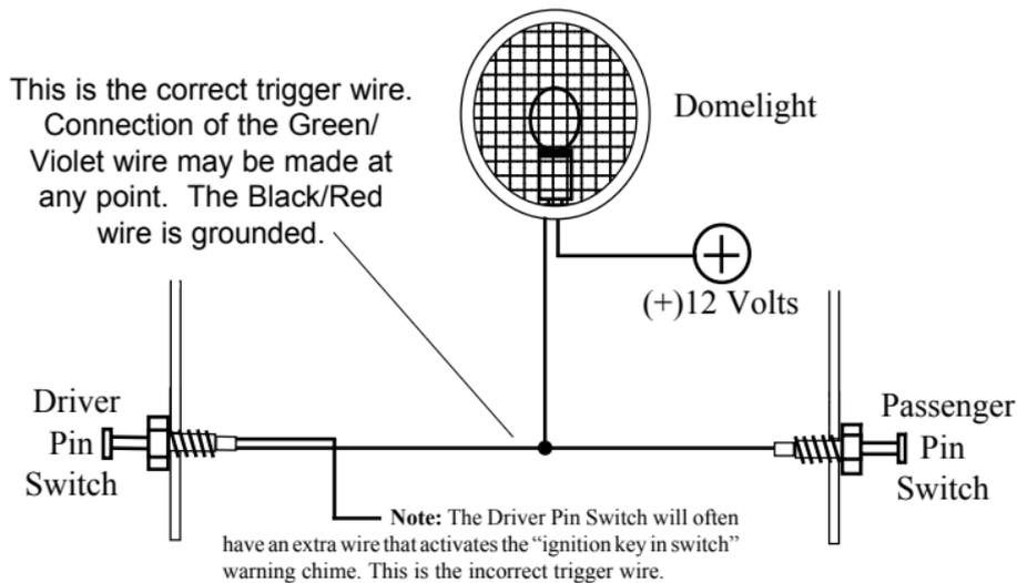
The **Violet** wire is identical to the Green Door Trigger wire, except that it is an open door input to the control module for vehicles having *Positive 12 volt* door pin switches.
