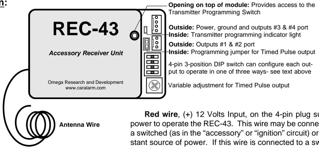
**Red wire**, (+) 12 Volts Input, on the 4-pin plug supplies power to operate the REC-43. This wire may be connected to a switched (as in the "accessory" or "ignition" circuit) or a constant source of power. If this wire is connected to a switched power source, the REC-43 will only operate when the source circuit is turned on (transmitter codes and output settings will not be affected).
