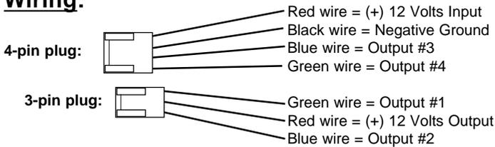
the application. When the REC-43 is used to operate other controlling devices (remote engine starter, for example), connection is typically wire-to-wire directly to the device's activation wire. The other most common interface method is connecting the output wire to activate a relay to control the vehicle's circuit (an example would be locking or unlocking the doors).
